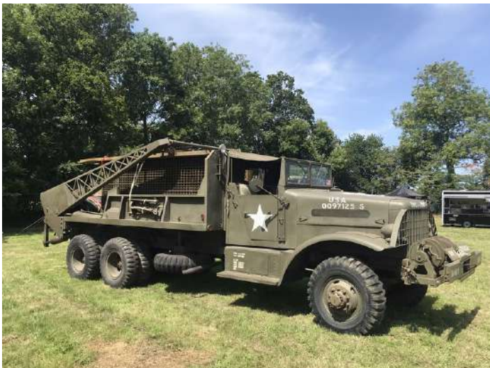
A Brockway truck for bridge construction
