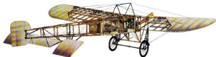
Blériot Type XI. The single-engine tractor propeller aircraft is the first plane to feature a modern structure : a monoplane with cruciform tail surfaces at the rear, with wings on either side of the cockpit. 800 units were built in 16 different models.
