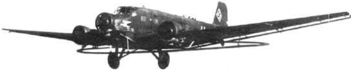
Junkers Ju-52 MS "Mausi". A total of approximately 70 Ju 52/3m were converted to the version "MinenSuch" (Minesweepers).
