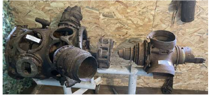
Parts of a BMW 801 D-2 engine from a German FW 190 fighter.
